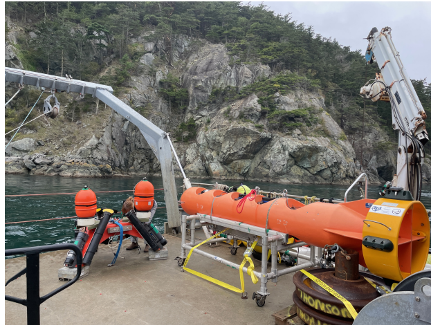
Figure 2: Sea Spider seafloor tripod and Stablemoor sub-surface buoy just before deployment. The shoreline of Blakely Island at the end of survey line 3 is just behind the vessel (100 m stand-off distance).
