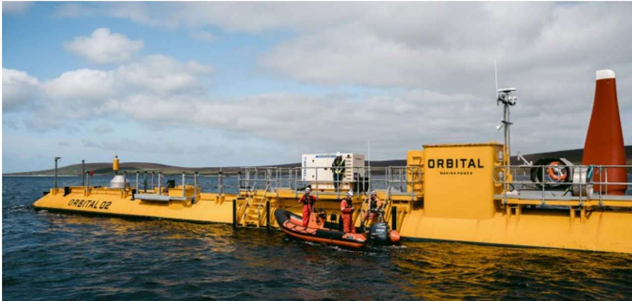
Figure 2. Orbital O2-X Deployment in Orkney Islands, Scotland (Wings Down – Operation)
