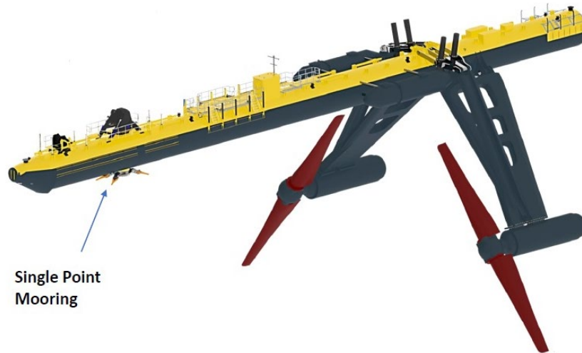
Figure 9. Single-Point Mooring Location on Orbital O2-X Hull
