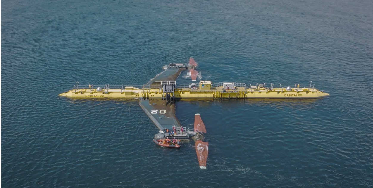
Figure 1. Orbital O2-X Deployment in Orkney Islands, Scotland (Wings Up - Standby)
