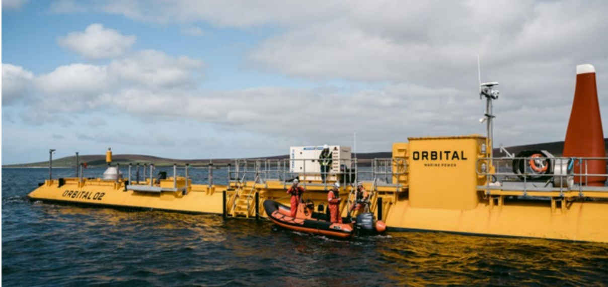
Figure 74. Example of Maintenance Personnel and Boat for Orbital Tidal Device
