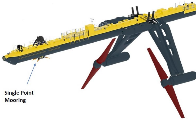
Figure 7. Single-Point Mooring Location on Orbital O2-X Hull
